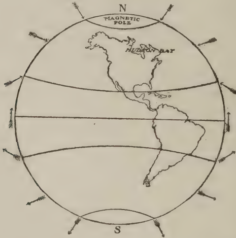
DIP OF THE MAGNETIC NEEDLE IN VARIOUS LATITUDES
